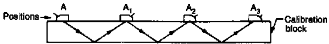
(a) Probe position on calibration block
